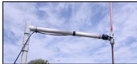
Dipole for 2m VHF - 38" tip to tip
