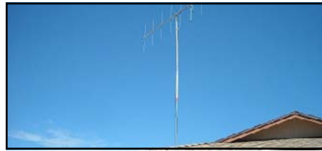
Beam aimed North to Phoenix - VHF 2meters
